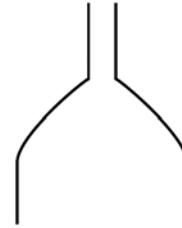
When the top of the blade slopes to the sides at an angle, the boot simply slides off preventing any energy from being transferred from the foot to the shovel. This wastes energy and causes the shoveler to become discouraged.
